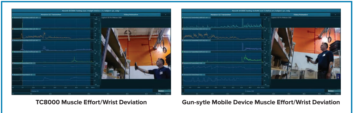
FIGURE 13: Muscle effort and wrist posture levels shown in the images below re-confirm the results in Phase 2 — amplitude of muscle signals and wrist deviations for scan and verify tasks is greatly reduced, resulting in faster task completion times.
